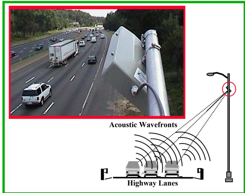
**Figure 1 SmarTek Systems Acoustic Sensor (SAS-1)**
