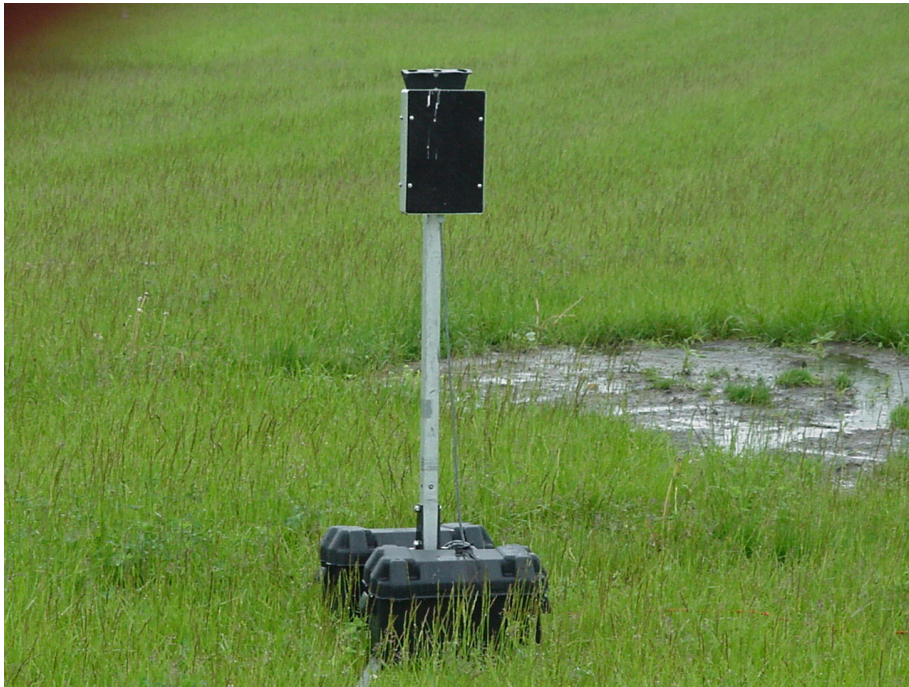
Front view of SAS-1 with battery pack base in Ames, Iowa demonstration
