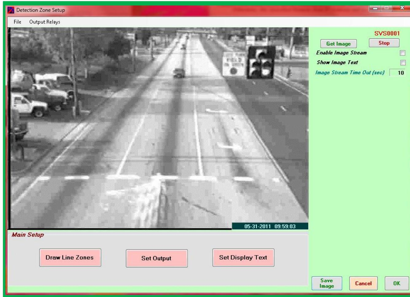
When setting up an SVS-1 camera channel for detection, the user should proceed by first **Drawing Line Zones**, then **Setting LZ Parameters**, then **Setting Detector Output**, and finally **Setting the descriptive text for the Output Video Display**. Click **Draw Line Zones** button.
