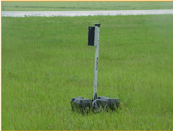
SAS-1 with battery pack base in Ames, Iowa demonstration
